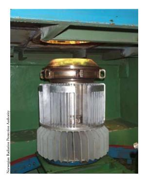
Radioisotope thermoelectric generator.
