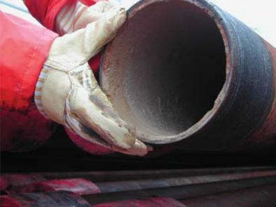
▲ Exposure to naturally occurring radioactivity can be enhanced as a result of TENORM industries, including oil and gas development. Scale on the inside of pipes can reach high levels and pose a hazard to workers. per kilogram. Procedures are commonly in place for protection of workers. Controls for the management of the waste arising, e.g. from pipe-cleaning operations, are necessary to protect the environment from contamination.
