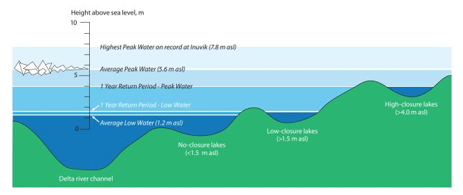
Figure 6.20. Classification of lakes in the Mackenzie River delta according to the extent of their isolation from the river. Ice-jam floodwaters are responsible for flooding of the riparian lake systems more hydraulically unconnected to the main flow system. Source: after Emmerton et al. (2007).
