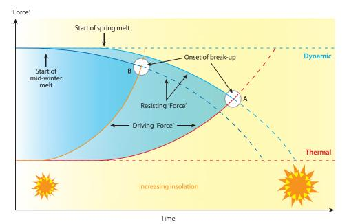
Figure 6.13. Schematic illustration of driving and resisting factors leading to different types of riverice break-up events. Point A refers to a spring break-up and point B to a mid-winter event with smaller decreases in ice resistance because of lower levels of incoming solar radiation. Adapted from Beltaos (1982).
