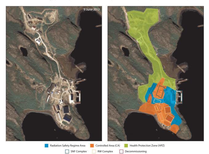
Figure 3.2 View of the Andreeva Bay STS site in 2013, showing the extent of the Radiation Saftey Regime, Controlled Area and Health Protection Zone. Main facilities at Andreeva Bay STS comprise the spent nuclear fuel (SNF) complex, the site of decommissioning operations, the radioactive waste (RW) complex, various supporting facilities and Pier PMK-67 (modified from Sneve et al. 2014).
