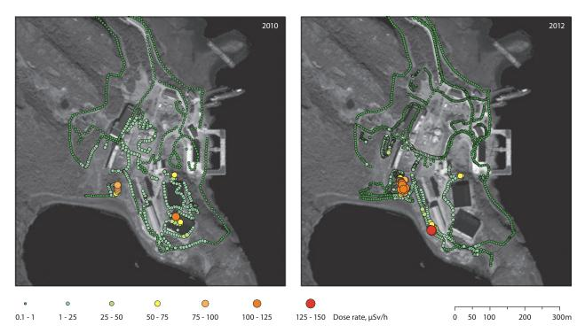
Figure 3.3 Gamma dose rate measurement routes at Andreeva Bay STS made by the Federal Medical-Biological Center (FMBC) of Russia in cooperation with SevRAO in 2010 and 2012 (Sneve et al. 2014).
