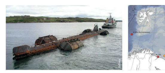
Figure 3.8 Nuclear submarine *K-159* under tow and the location at which it sank. The map shows the location of *K-159* and other sunken nuclear submarines in the Barents region, *K-27* (Sect. 4.5.1), *K-278* (Sect. 2.2.4) and *K-141* (*Kursk*, now raised).
