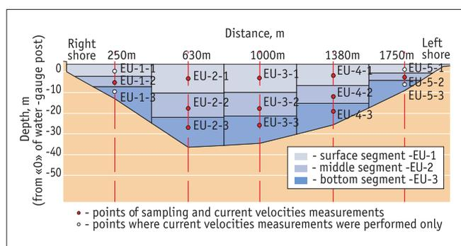
Figure 4.43. Channel profile and sampling/measurement points on the Yenisey river at the downstream cross-section near Ust'-Port.
