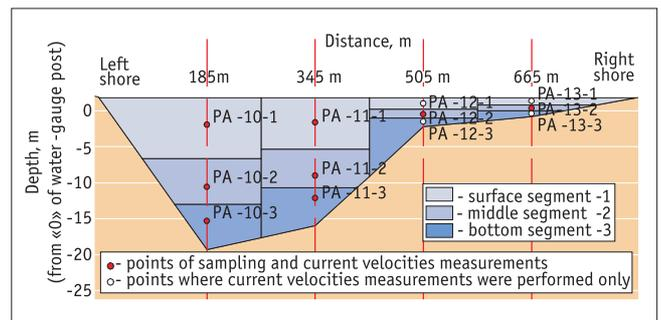
Figure 4.41. Channel profile and sampling/measurement points on the Small Pechora river at the downstream cross-section near Andeg settlement.
