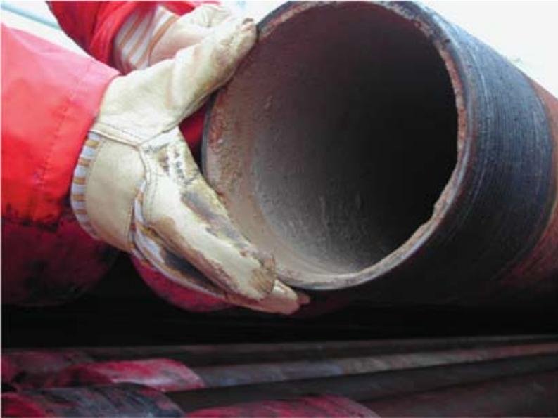
▲ Exposure to naturally occurring radioactivity can be enhanced as a result of TENORM industries, including oil and gas development. Scale on the inside of pipes can reach high levels and pose a hazard to workers.
