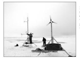
Figure 9. Deployment of a remote weather station. Batteries charged by solar panels and a wind generator, seen in the fore-ground, powered the instruments.
