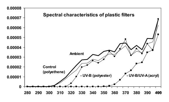
Fig. 1(b). Spectral characteristics of the plastic filters used in the experiment.
