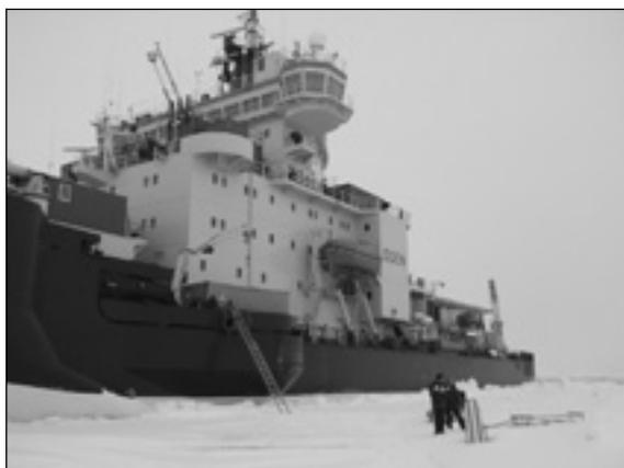
Figure 3. Side view of *Oden* showing the 4th deck row of laboratory containers with the masts for air intakes.
