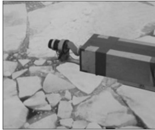
Figure 6. Scanning microwave radiometer mounted on the starboard side of the 7th deck, with a free view over the ocean.
