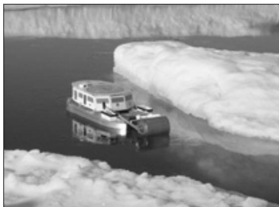
Figure 4. The remote controlled miniature boat used to sample the ocean surface micro-layer.
