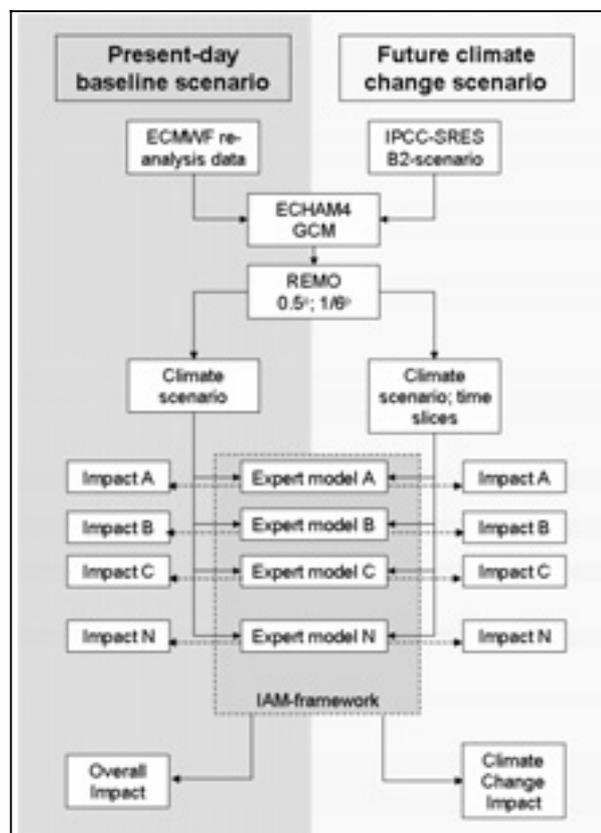
Figure 2: Basic components of the BALANCE-IAM and modelling strategy
