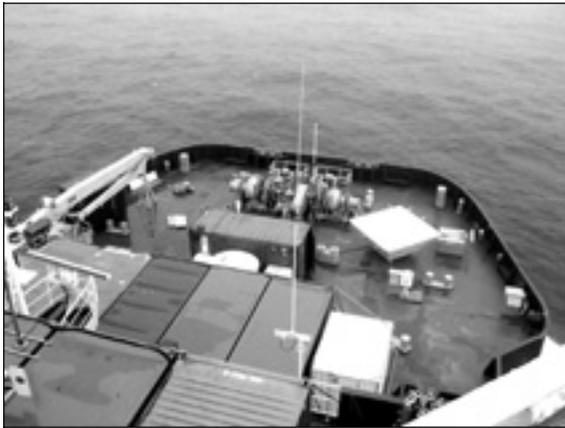
Figure 5. View of the *Oden* foredeck from the 7th deck, showing the square-shaped NOAA/ETL 915MHz Wind Profiler antenna and the round S-band cloud radar antenna, also from NOAA/ETL, partly hidden aft of the forward container housing electronics for both systems.
