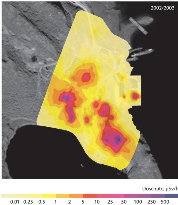
Figure 3.4 Interpolated dose rate levels at 1 m above ground level from measurements made in 2002–2003 across the Andreeva Bay STS site (Reistad et al. 2008). Note the log scale.
