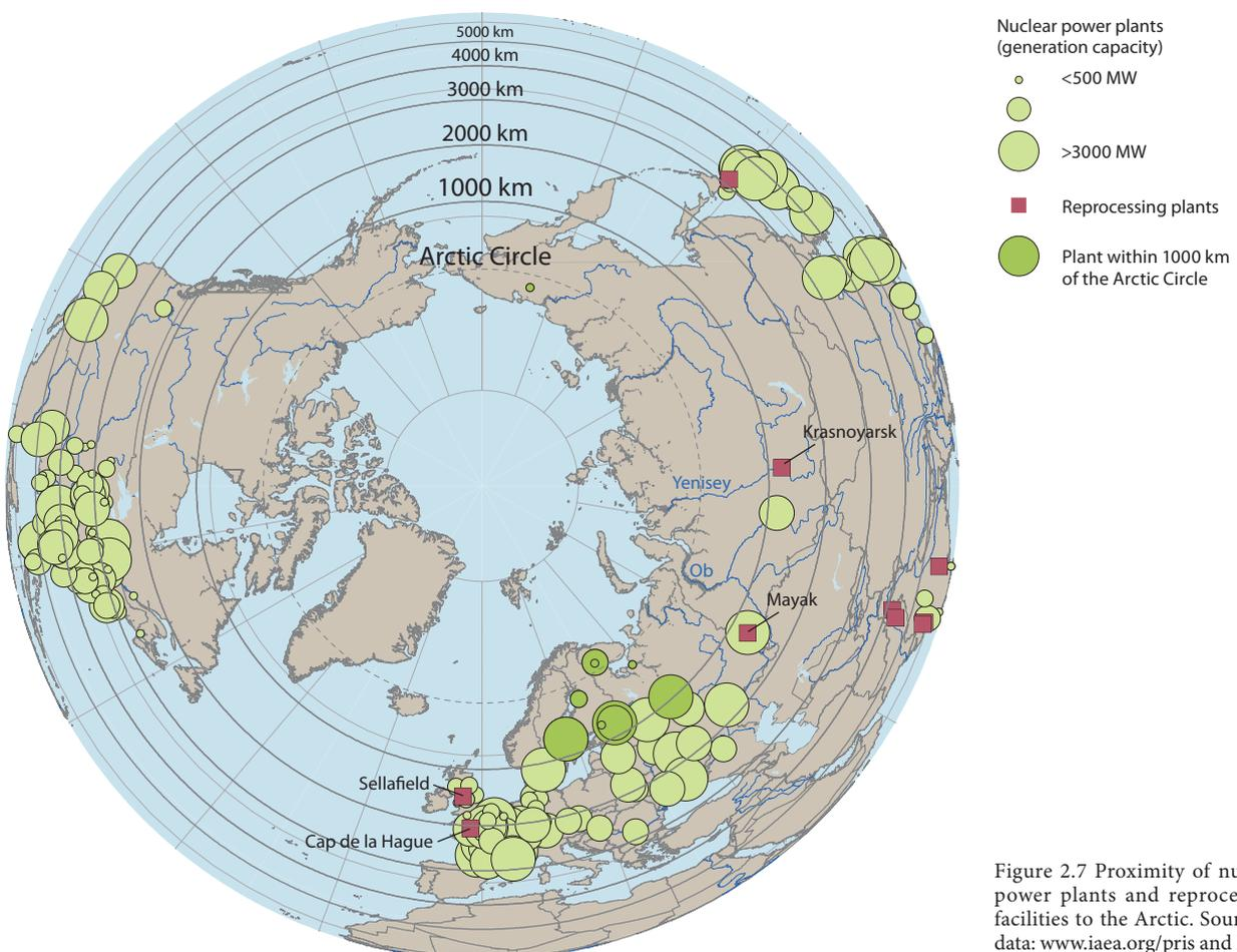
Figure 2.7 Proximity of nuclear power plants and reprocessing facilities to the Arctic. Source of data: [www.iaea.org/pris](http://www.iaea.org/pris) and Davis et al. (2015).
