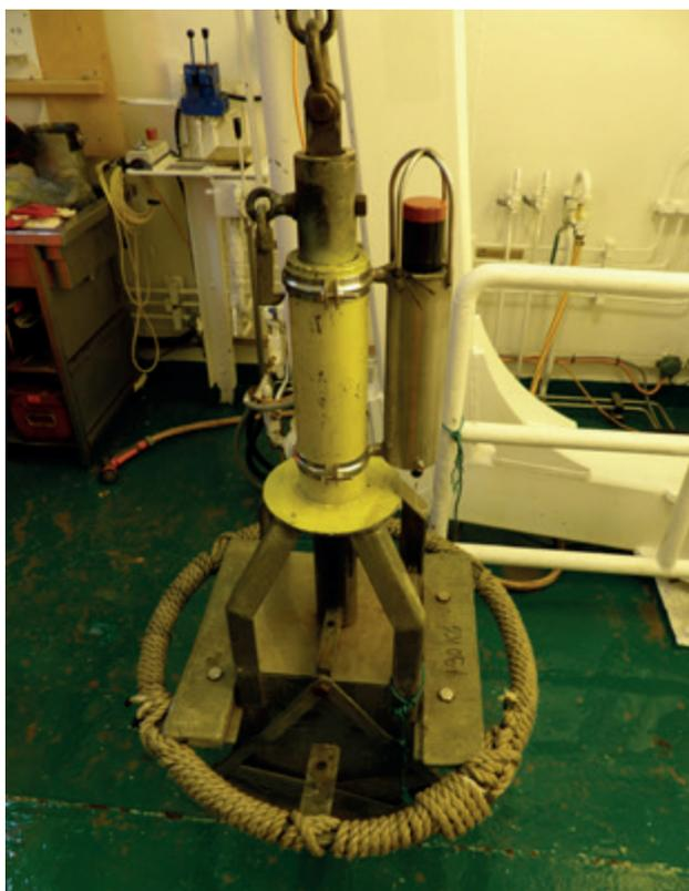
Figure 2.3 An acoustic transponder attached to the sediment grab allowed precise sediment sampling with regard to the position of the sunken *Komsomolets* submarine.
