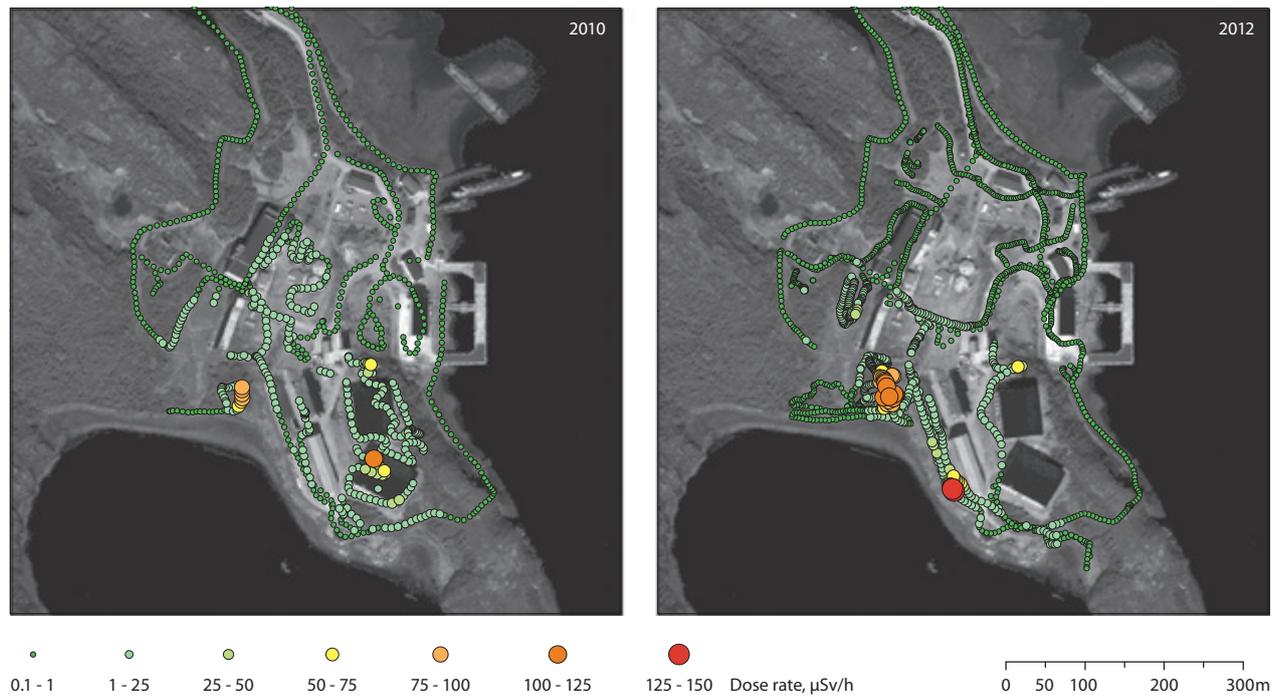
Figure 3.3 Gamma dose rate measurement routes at Andreeva Bay STS made by the Federal Medical-Biological Center (FMBC) of Russia in cooperation with SevRAO in 2010 and 2012 (Sneve et al. 2014).
