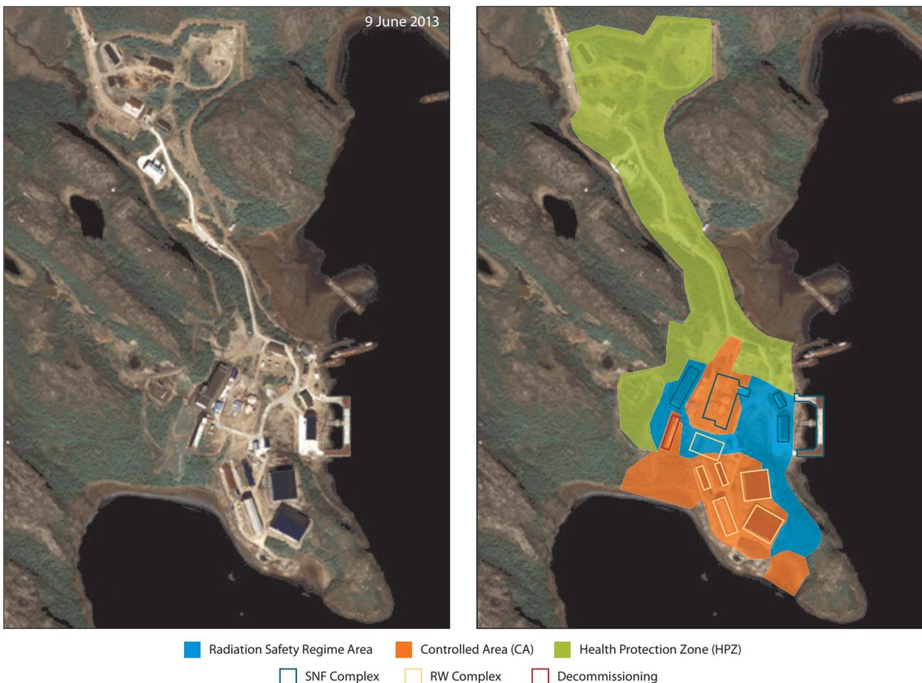
Figure 3.2 View of the Andreeva Bay STS site in 2013, showing the extent of the Radiation Safety Regime, Controlled Area and Health Protection Zone. Main facilities at Andreeva Bay STS comprise the spent nuclear fuel (SNF) complex, the site of decommissioning operations, the radioactive waste (RW) complex, various supporting facilities and Pier PMK-67 (modified from Sneve et al. 2014).
