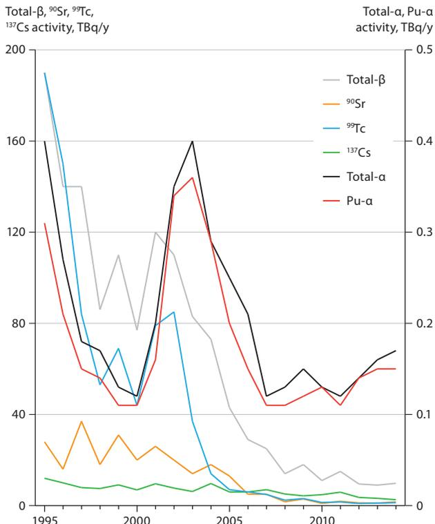
Figure 2.4 Annual discharges of selected radionuclides to the Irish Sea from the Sellafield nuclear fuel reprocessing plant (OSPAR 2007, 2008, 2009, 2010, 2011, 2012, 2013, 2014).
