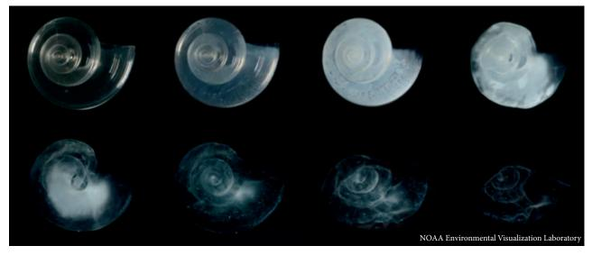
In laboratory experiments, this pterapod shell dissolved over the course of 45 days in seawater adjusted to an ocean chemistry projected for the year 2100.
